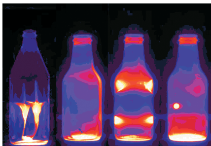
▲ Fig 2. Examples of defects: Birdswings, blisters and inclusions.
