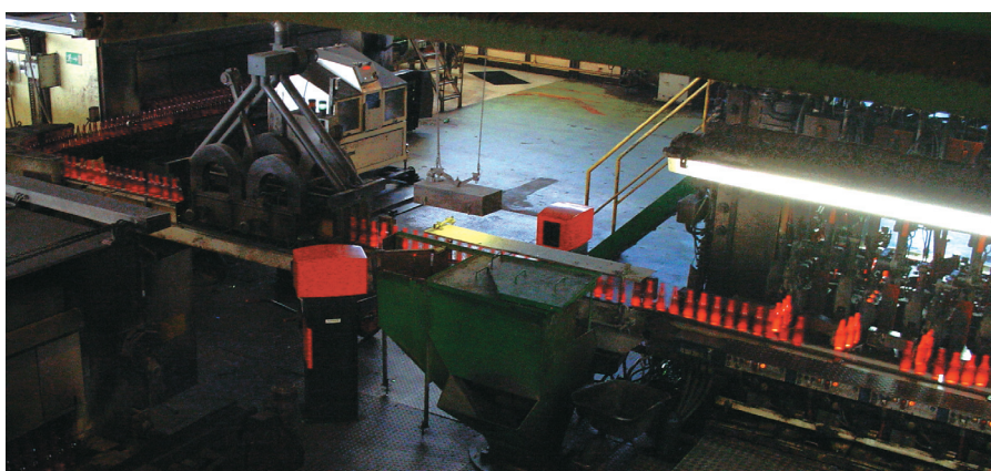
▲ Fig 1. Xpar Vision's hot end infra-red camera system for inspection and process monitoring and control.
